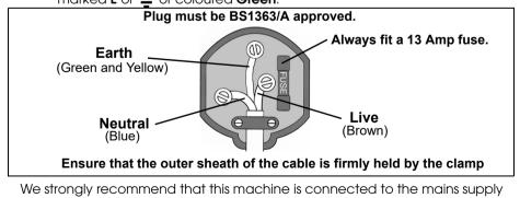
We strongly recommend that this machine is connected to the mains supply via a Residual Current Device (RCD). If in any doubt, consult a qualified electrician. DO NOT attempt any repairs yourself.
