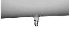
5. When the reservoir has been drained, re-tighten the vent valve and remove the hose.
